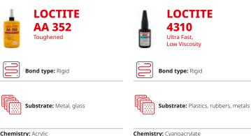
Chemistry: Acrylic Viscosity: 20,500 mPa·s Compliant with ISO 10993: No Fluorescence: No Colour: Clear/light amber Use with: LOCTITE SF 7649 Activator Chemistry: Cyanoacrylate Viscosity: 175 mPa•s Compliant with ISO 10993: Yes Fluorescence: Yes Colour: Clear/pale green
