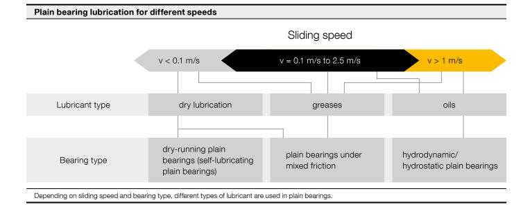
Continuous operation with low wear and minimum friction during start-up and slow-down are the prerequisites of hydrodynamic plain bearings offering full performance. Oil-lubricated plain bearings will only attain their specified service life if the correct lubricant and required viscosity are used.
