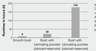
$\label{eq:p} \begin{array}{l} p = 23 \ \text{N/mm}^2 \\ \text{Oscillating angle} = 60 \ ^{\circ}\text{C} \\ \text{v}_{\text{m}} = 0.05 \ \text{m/s} \\ \text{Ambient temperature} \\ \text{Steel shaft} \\ \text{Bronze plain bearing made by Wieland Werke Ulm,} \\ \text{preferably lubricated with Klüberplex SK 12} \end{array}$
