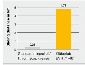
Temperature: ambient Bearing temperature: 40 to 60 °C  $p = 50 \text{ N/mm}^2$ v = 0.01 m/sPlain bearing: CAROBRONZE Shaft: rotating, steel 1.3349, hardness 46HRC, roughness Rz 2.5 Test is terminated when the friction value  $\mu > 0.2$
