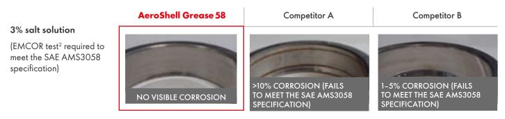
Meeting the specifications where others fail: AeroShell Grease 58 exceeds SAE AMS3058 corrosion requirements. Not all the popular, lithium-complex wheel-bearing greases meet these specifications or protect against the effects of the latest runway de-icing fluids. AeroShell Grease 58 is also better than or equals competitors' products in EMCOR tests with corrosive runway de-icing fluids, thereby offering the best overall corrosion protection.
