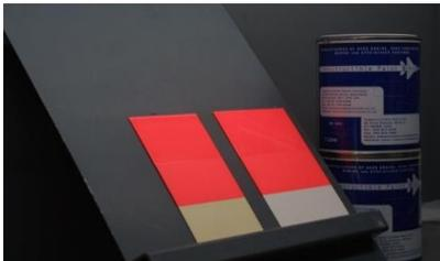
2-3 coat system for metals and composites featuring matt white epoxy basecoat, fluorescent or luminescent polyurethane colour coat, and, where required, polyurethane clear gloss glaze coat.
