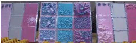
Paint stripper applied
