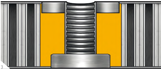
1 Inserts on honeycombs assembly 2 Inserts with A 140 3 Inserts
