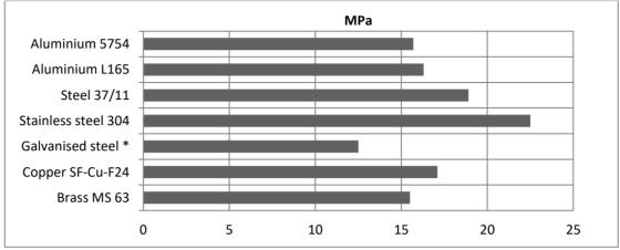
Cured 16 hours at 40 °C and tested at 23 °C. Pretreatment: sandblast + degrease
