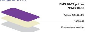
\* For B787 a/c. Intermediate coat (optional): Follow OEM recommendation / Re-fresh primer: Follow OEM recommendation / Structural repair etc.: Follow substrate preparation
