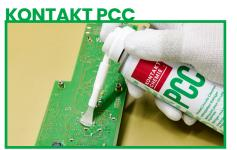
After soldering printed circuit boards, flux residues do not only look unaesthetic, but can also cause corrosion damage and electrical breakdown by leakage currents.
