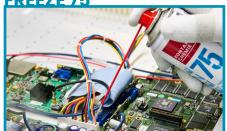
Cooling spray. Intermittent short circuits or interruptions in condensers and resistors are quickly discovered with FREEZE 75.
