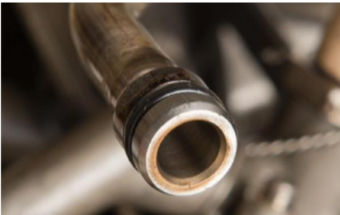
Sealing rings in excellent condition throughout, including this oil spray nozzle
