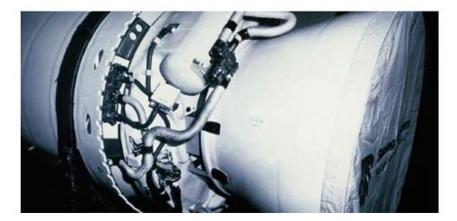
Nextel Ceramic Fabric is a key component in the development of strong, lightweight space debris shields, for use on the Space Station Laboratory Habitation and other U.S. manned (e.g. ISS) and unmanned missions (e.g. Stardust Mission).
