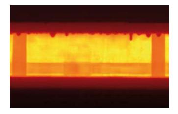
Lift gate in a sinter metal production furnace with  $H_2/N_2$ -atmosphere at 1,300 °C.
