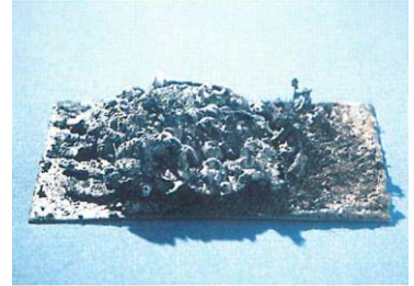
Panel a - showing depth of "char" created after 5 minutes flame exposure.
