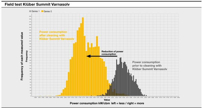
The field test shows that power consumption decreased by  $5\,\%$  on average when using Klüber Summit Varnasolv
