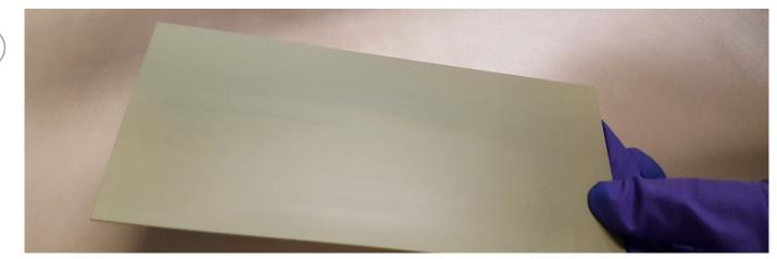
After application of the adhesion promoter, place the parts in a clean environment and allow them to dwell for at least 30 minutes, or as recommend on the relevant adhesion promoter technical data sheet or process specification. After the dwell time, sealant can be applied directly over the areas treated with adhesion promoter.
