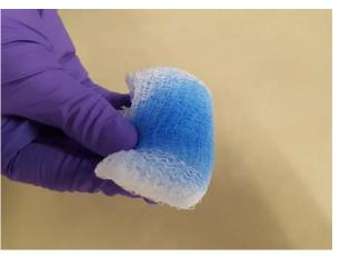
Lightly wet a clean gauze pad or AMS3819 wipe with the adhesion promoter. The gauze or pad should be moist, but not soaked or dripping wet.
