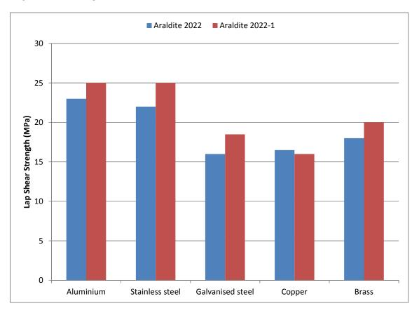
Substrates: sandblasted & degreased with acetone
