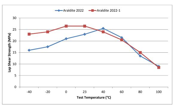
Lap Shear Strength vs temperature (ISO 4587)
