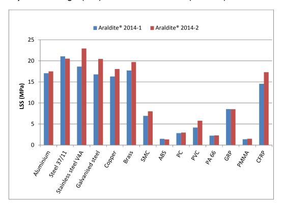
Metal substrates : sandblasted & degreased with acetone Plastic substrates : abraded & degreased with isopropanol
