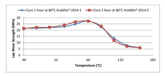
Tg measurement (24h at RT + 1h at 80°C curing)
